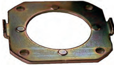
139936 Bearing Plate Replacing: 021411-0450 Servicing: 100211-1000, 100211-1001, 100211-1010, 100211-1011, 100211-1020, 100211-1021, 100211-1030, 100211-1031, 100211-1040 ID 34.00, OD 52.50x52.50, Thickness 1.70, Dist. mount. holes 38.00, No./mount. holes 4 Bearing: O.D. 46.00 mm.
