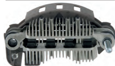
236559 Rectifier Replacing: RM-154HV, 31127-PGM-004 Servicing: 31100-PND-004, A002TB7591, A002TB8691, A002TC0691, A002TC0691A, A002TC0691AE, A002TC0691ZE, A2TB7591, A2TB7951 B+ M6, B+/threaded M6/24.53, ID 28.00, OD 99.00, Mount. dist. 85.00, B+ type Bolt, No./diodes 8, Capacitor w/ Alternative no.: 333823
