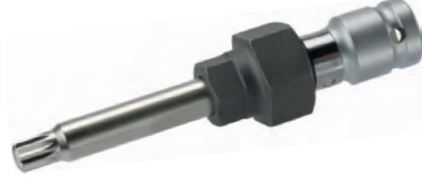
211081 Combi Tool Servicing: Valeo For removing and installing of rubber clutch pulley. XZN 10.00x128.00 mm w/ 1/2" socket and 28.00/19.00 mm hexagon.
