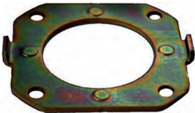
139935 Bearing Plate Replacing: 021411-0400 Servicing: 100211-1000, 100211-1001, 100211-1010, 100211-1011, 100211-1020, 100211-1021, 100211-1030, 100211-1031, 100211-1040 ID 32.00, OD 49.00x49.00, Thickness 1.60, Dist. mount. holes 35.00, No./mount. holes 4, Gasket w/o Bearing: O.D. 43.00 mm.
