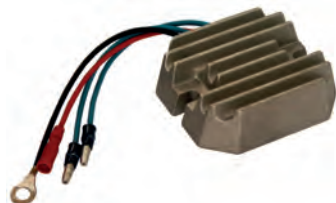
234409 Regulator/Rectifier Replacing: RS1104 14 Volt, Dist. mount. holes 64.25 Terminals: -(black), B+(red), AC(blue), AC(blue).
