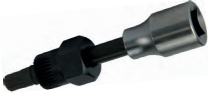
210843 Combi Tool Servicing: Bosch Alternators 33 teeth combitool for the disassembly and assembly of the free wheel pulley. XZN 10.00x110.00 mm, w/ 1/2" socket and 22.00 mm hexagon.
