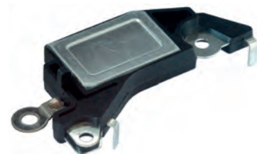
138387 Regulator Replacing: 273310, 273110 Servicing: 102203500, 102203510, 219072, 219081 28 Volt, 27.7 Volt setting, Dist. mount. holes 65.50, Regulator type Electronic
