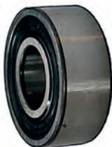
140900 62203-2RS1/C3 Ball Bearing Manufacturer: SKF ID 17.00, OD 40.00, Height 16.00
