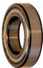
140887 FAG 6007-2ZR Ball Bearing ID 35.00, OD 62.00, Height 14.00
