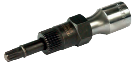
210909 Combi Tool Servicing: Valeo Alternators 33 teeth combitool for disassembly and assembly of free wheel pulley. Torx 50.00x110.00 mm, w/ 1/2" socket and 22.00 mm hexagon.
