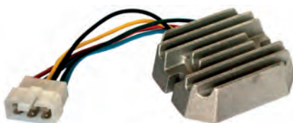
234413 Regulator/Rectifier Replacing: RS5104, RS5102 14 Volt, Dist. mount. holes 61.20 Terminals: AC(blue), -(black), AC(blue), L(green), IG(yellow), B+(red).
