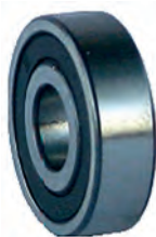
141058 609-2RS/C3 Ball Bearing ID 9.00, OD 24.00, Height 7.00
